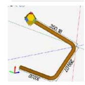
**Designer - Template Advanced:** The Template Advanced group includes dozens of predefined shapes of the most commonly bent tubes. The user simply enters the dimensional values into the templates fields and the part is created. Many of the templates include outside and inside line of material for sizing along with the standard center line.
