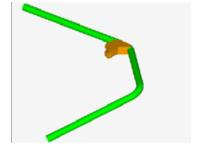
**Plug-in - Manufacture Checking:** Setup minimum length distance in your die description for the first straight length, the distance between bends, and the last or holding straight leg length. This is not collision checking but does offer a quick check to make sure the part has enough material between bends to be successful.
